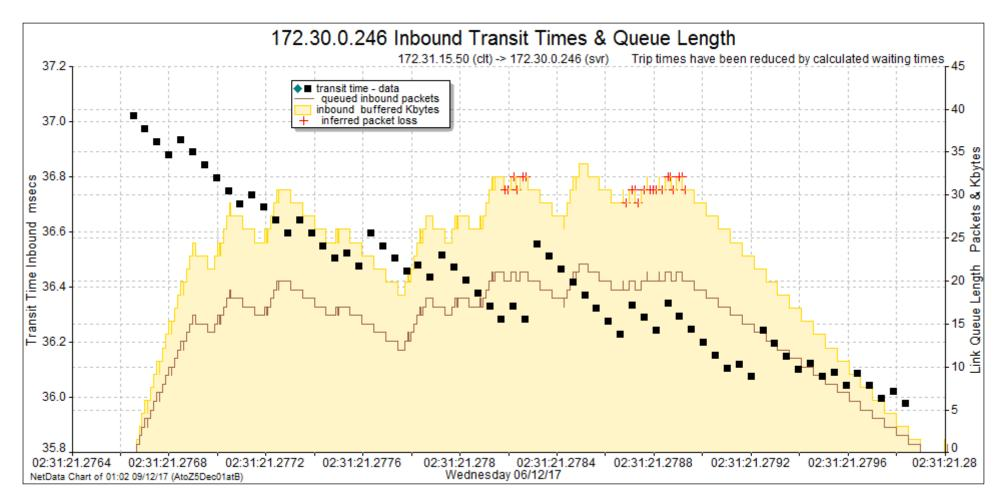
In another model, if packets arrived in a router at 1 Gbps and queued for egress at 250 Mbps, then the lost packets would have been discarded when the queue held 20 packets (30 KB), but some successful packets would have to wait for one millisecond.
