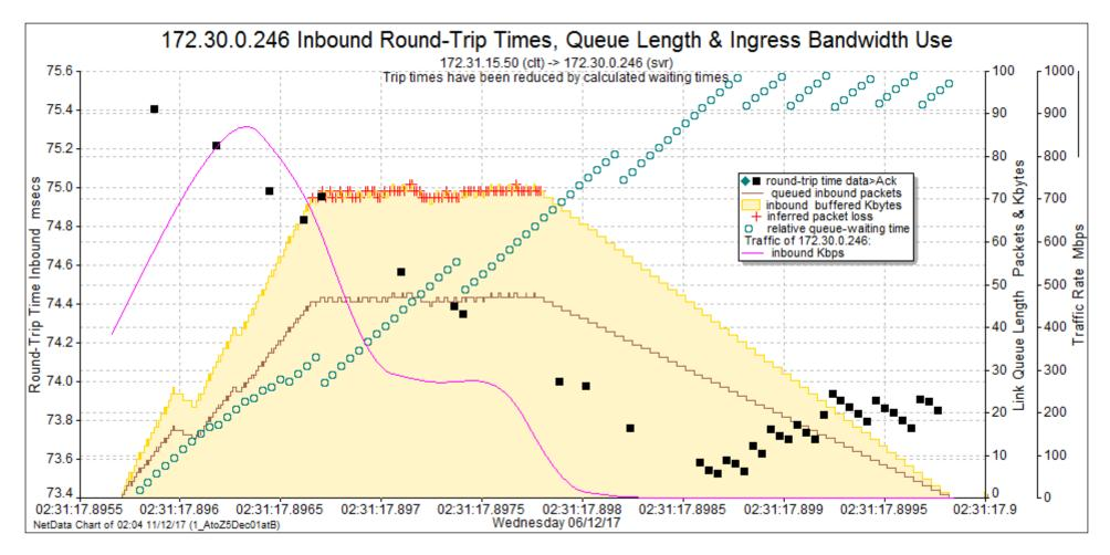
A model of the packet queue between a 1 Gbps link and a 280 Mbps link formed by the first packet burst that suffered packet loss indicated that packets would have been dropped when the queue had 45 packets and occupied 70 KB (RHS scale, red and yellow lines).
