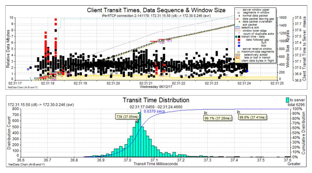
On the top chart, the black squares represent the measured trip times for each packet as measured by comparing the "At B" and "At Y" after adjusting the time stamps. The scale is on the RHS and we see that the variation is mostly between 36.85 and 37.30 ms (0.45 ms). The red squares are packets that followed a gap and it is only for those that we see more significant delays of an additional 0.4 ms (as if the packet loss mechanism also involves a small amount of queueing).
