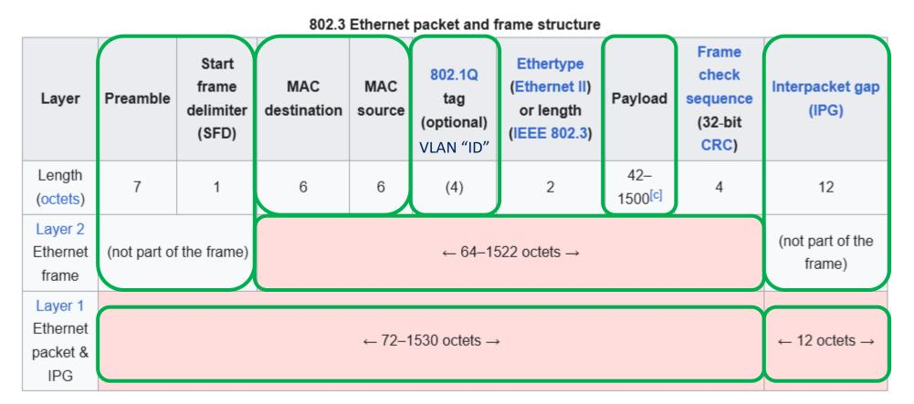
The optional 802.1Q tag consumes additional space in the frame. Field sizes for this option are shown in brackets in the table above. IEEE 802.1ad (Q-in-Q) allows for multiple tags in each frame. This option is not illustrated here.
